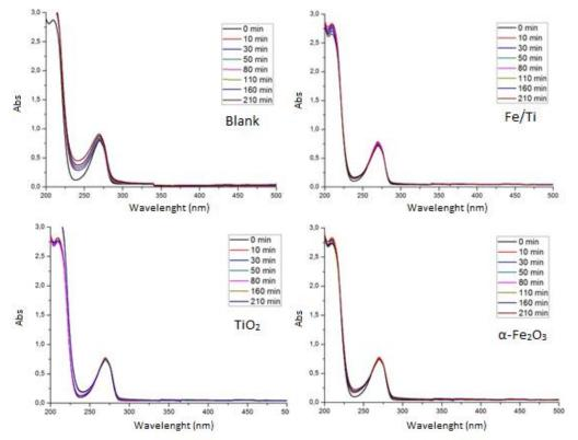
**Figure 3:** Absorption espectra during the heterogeneous photo-Fenton test ( $C_{H2O2}=100$ mg.L<sup>-1</sup>;  $C_{phenol}=50$ mg.L<sup>-1</sup>;  $C_{catalystr}=0.1$ g.L<sup>-1</sup> and pH=6.5), with (a) TiO<sub>2</sub>, (b) Blank, (c)  $\alpha$ -Fe<sub>2</sub>O<sub>3</sub> and (d) mixed oxide Fe/Ti
