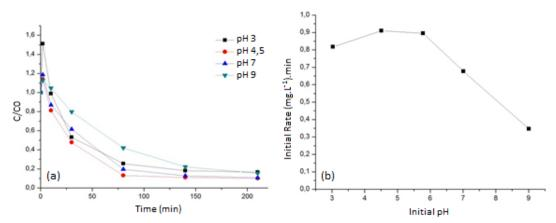
**Figure 8:** (a) Phenol removal for different initial pH of solution, with  $0.1g.L^{-1}$  Fe<sub>2</sub>O<sub>3</sub>-TiO<sub>2</sub>, 50mg.L<sup>-1</sup> phenol and 100mg.L<sup>-1</sup> H<sub>2</sub>O<sub>2</sub> (b) initial rate of reaction *versus* initial pH of solution
