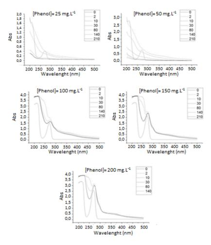
**Figure 11:** Absorption spectra of phenol solutions during the phenol variation test  $(C_{H2O2}=100 \text{ mg/L}; C_{catalyst}=0.050 \text{ g/L e pH}\cong6)$ , with different phenol concentrations.
