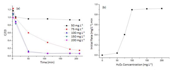
**Figure 6:** (a) Phenol removal for different  $H_2O_2$  concentrations, with  $0.1g.L^{-1}$  Fe<sub>2</sub>O<sub>3</sub>-TiO<sub>2</sub>, 50mg.L<sup>-1</sup> phenol, and initial pH=6 and (b) initial rate of reaction *versus*  $H_2O_2$  concentration
