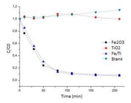
**Figure 4:** Performance comparison of the mixed oxide, hematite, titanium dioxide and blank (without catalyst). The following initial conditions were used:  $C_{H2O2}=100$ mg.L<sup>-1</sup>;  $C_{phenol}=50$  mg.L<sup>-1</sup>;  $C_{catalyst}=0.1$ g.L<sup>-1</sup> and pH $\cong$ 6.5.
