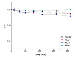
Figure 2: Efficiency for each catalyst at time intervals of 0 to 210 min
