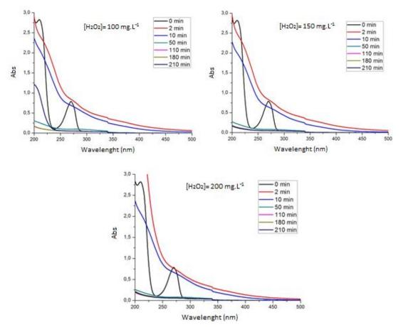
**Figure 5:** Absorption spectra of phenol solutions during the hydrogen peroxide variation test  $(C_{phenol}=50 \text{mg.L}^{-1}; C_{catalyst}=0.1 \text{g.L}^{-1} \text{ and } \text{pH}\cong5.8)$ , variating H<sub>2</sub>O<sub>2</sub> concentration.
