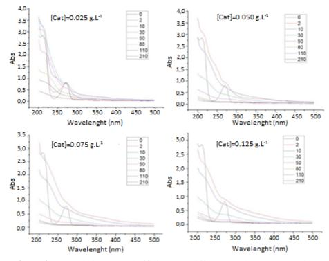
Figure 9: Degradation phenol efficiency at different catalyst concentrations.
