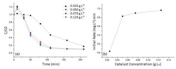
**Figure 10:** (a) Phenol removal for different  $Fe_2O_3$ -TiO<sub>2</sub> concentrations, with 50mg.L<sup>-1</sup> phenol, 100mg.L<sup>-1</sup> H<sub>2</sub>O<sub>2</sub> and initial pH=6 and (b) initial rate of reaction *versus* catalyst concentration
