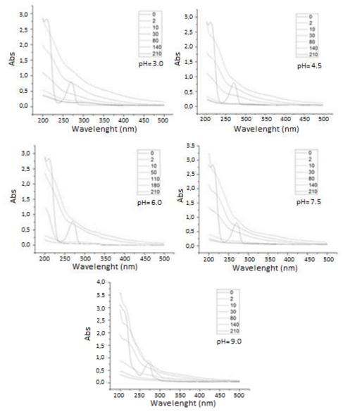
**Figure 7:** Absorption spectra of phenol solutions during the pH variation test ( $C_{H2O2}=100$ mg.L<sup>-1</sup>,  $C_{phenol}=50$  mg.L<sup>-1</sup> and  $C_{catalyst}=0.1$ g.L<sup>-1</sup>) variating the initial solution pH.
