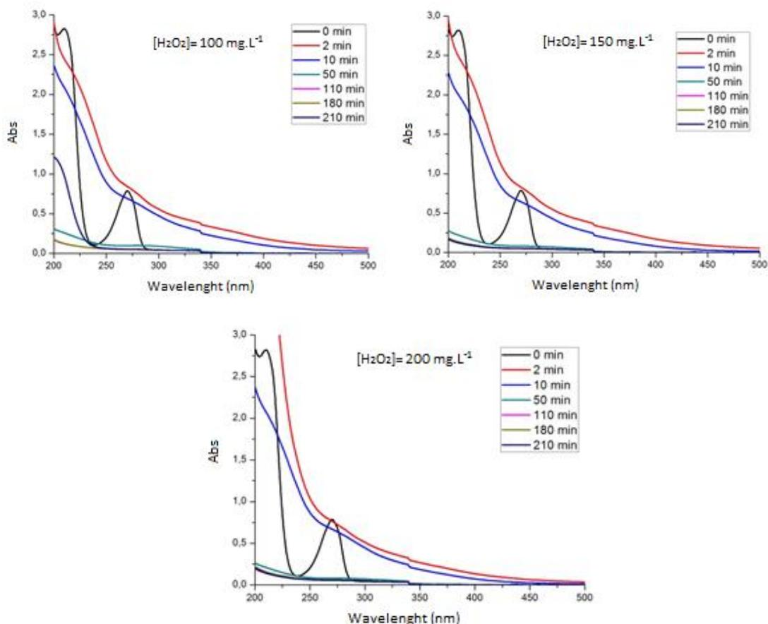
**Figure 5:** Absorption spectra of phenol solutions during the hydrogen peroxide variation test ( $C_{\text{phenol}}=50\text{mg.L}^{-1}$ ;  $C_{\text{catalyst}}=0.1\text{g.L}^{-1}$  and  $\text{pH}\cong 5.8$ ), varying  $\text{H}_2\text{O}_2$  concentration.
