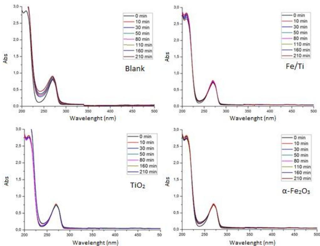
**Figure 3:** Absorption spectra during the heterogeneous photo-Fenton test ( $C_{\text{H}_2\text{O}_2}=100\text{mg.L}^{-1}$ ;  $C_{\text{phenol}}=50\text{mg.L}^{-1}$ ;  $C_{\text{catalyst}}=0.1\text{g.L}^{-1}$  and  $\text{pH}=6.5$ ), with (a)  $\text{TiO}_2$ , (b) Blank, (c)  $\alpha\text{-Fe}_2\text{O}_3$  and (d) mixed oxide Fe/Ti
