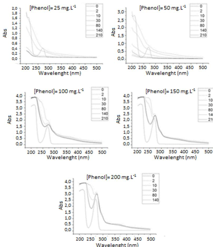
**Figure 11:** Absorption spectra of phenol solutions during the phenol variation test ( $C_{H_2O_2}=100\text{mg/L}$ ;  $C_{\text{catalyst}}=0.050\text{g/L}$  e  $\text{pH}\cong 6$ ), with different phenol concentrations.
