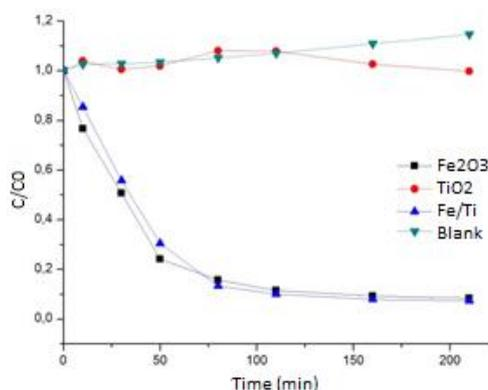
**Figure 4:** Performance comparison of the mixed oxide, hematite, titanium dioxide and blank (without catalyst). The following initial conditions were used:  $C_{H_2O_2}=100\text{mg.L}^{-1}$ ;  $C_{\text{phenol}}=50\text{mg.L}^{-1}$ ;  $C_{\text{catalyst}}=0.1\text{g.L}^{-1}$  and  $\text{pH}\cong 6.5$ .
