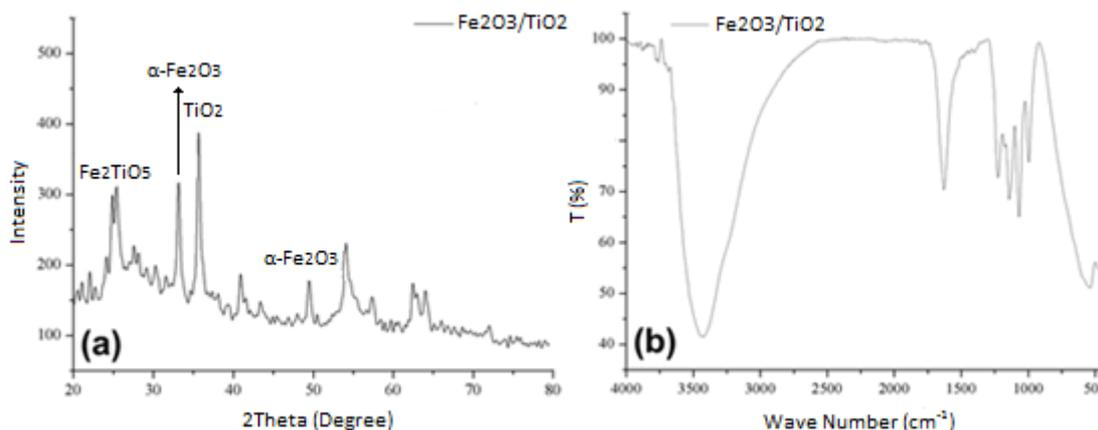
**Figure 1:** (a) X-ray diffraction patterns of Fe<sub>2</sub>O<sub>3</sub>/TiO<sub>2</sub> and (b) FT-IR spectra of Fe<sub>2</sub>O<sub>3</sub>/TiO<sub>2</sub>
