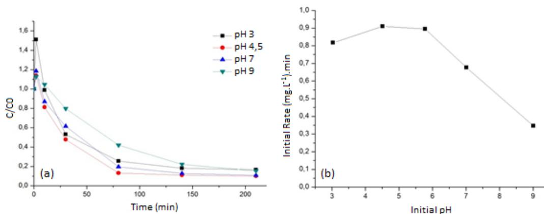
**Figure 8:** (a) Phenol removal for different initial pH of solution, with  $0.1\text{g.L}^{-1}$   $\text{Fe}_2\text{O}_3\text{-TiO}_2$ ,  $50\text{mg.L}^{-1}$  phenol and  $100\text{mg.L}^{-1}$   $\text{H}_2\text{O}_2$  (b) initial rate of reaction *versus* initial pH of solution
