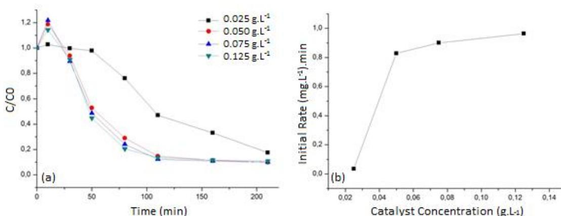
**Figure 10:** (a) Phenol removal for different  $\text{Fe}_2\text{O}_3\text{-TiO}_2$  concentrations, with  $50\text{mg.L}^{-1}$  phenol,  $100\text{mg.L}^{-1}$   $\text{H}_2\text{O}_2$  and initial  $\text{pH}=6$  and (b) initial rate of reaction *versus* catalyst concentration
