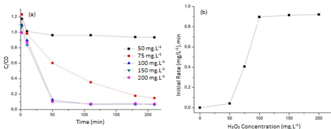
**Figure 6:** (a) Phenol removal for different  $\text{H}_2\text{O}_2$  concentrations, with  $0.1\text{g.L}^{-1}$   $\text{Fe}_2\text{O}_3\text{-TiO}_2$ ,  $50\text{mg.L}^{-1}$  phenol, and initial  $\text{pH}=6$  and (b) initial rate of reaction *versus*  $\text{H}_2\text{O}_2$  concentration
