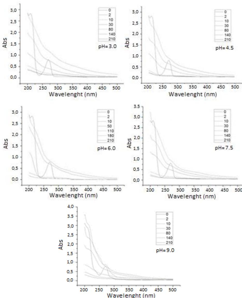
**Figure 7:** Absorption spectra of phenol solutions during the pH variation test ( $C_{H_2O_2}=100\text{mg.L}^{-1}$ ,  $C_{phenol}=50\text{ mg.L}^{-1}$  and  $C_{catalyst}=0.1\text{g.L}^{-1}$ ) varying the initial solution pH.
