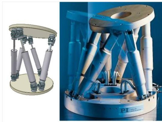
Fig. 5 Modern platform Stewart which uses only (18) couplings grade 4 (C4)
