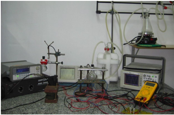
Figure 1 - Basic experimental scheme, a function generator, an amplifier, the variables coils, the resonator and the piezoelectric (PZT), and, in addition, the oscilloscopes
