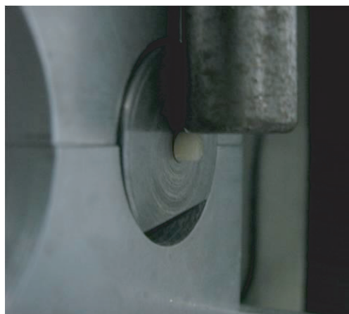
FIGURE 4 Shear test. Matrix with the specimen inside (A), attached to aluminum device (B), with the ceramic portion receiving the load of the active tip and flat device (C).
