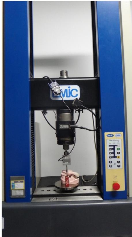
**Fig. 2.** EMIC testing machine (compressive forces applied).
