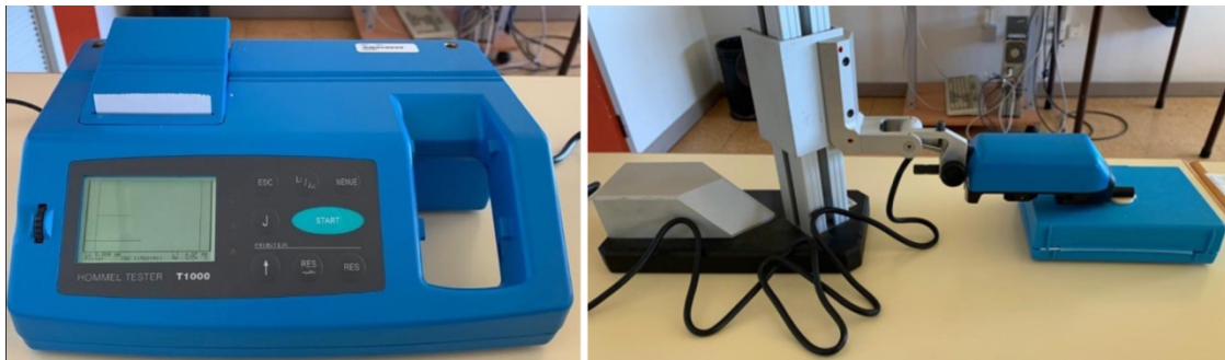
Figure 6. HOMMEL T1000® device used to obtain the measurements of surface roughness.
