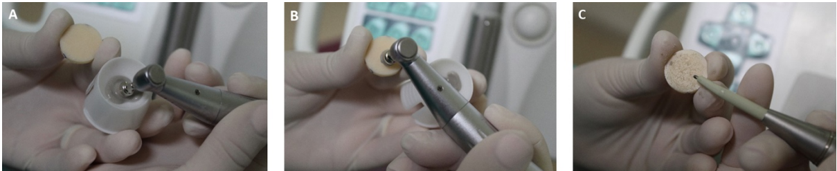
Figure 3. Polishing and finishing protocol with pumice paste. A. Impregnate the prophylactic brush with pumice paste; B. Application without water; C. Washing and drying with an air/water syringe.
